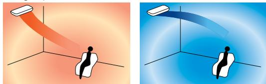
2. Saving energy, by preventing overcooling or overheating during night time by using the **night set mode**.
