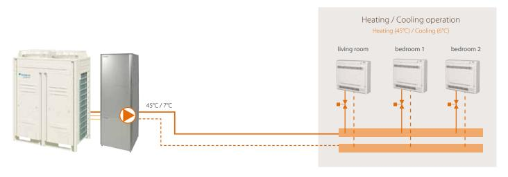
All type of heat emitters can be connected to Daikin Altherma Flex Type, thanks to its wide water temperature range. Daikin Altherma Flex Type is able to work with multiple set points, allowing a combination of different heat emitters operating at different water temperatures. The set point of the indoor unit will be lowered in function of the actual demand of the various heat emitters, ensuring optimum efficiency at all times and under all conditions.
